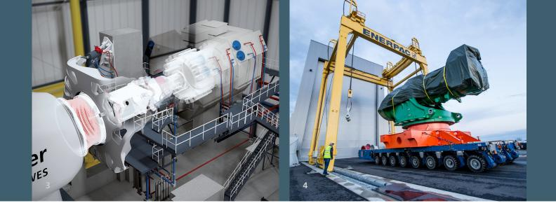
Here, wind load simulations can comprise of simulations from varying static and dynamic operating conditions as also from real-time simulation load data. In order to test wind energy turbines as comprehensively as possible, pitch systems as well as yaw systems can be integrated into turbine testing. For this purpose, individual system control values using actuators are implemented in real-time simulation.
